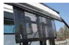
Window Screen Mounted to Tarp System Gantry
