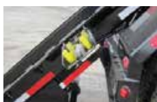
"The Hooker" Securement System at Rear Hinge
